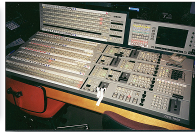
Figure 6.39 Sony DVS-7000 switcher control panel used for ABC's Monday Night Football. Each TD sets up their board based on their experience, the particular board, and the needs of the director and show. This photo shows another interesting facet of today's switchers. Notice that the various effects banks are labeled with different sources. Switchers today are also routers. These switchers can often input 64 or more inputs, many more than the 30 or 32 buttons now common per bank. Switchers today literally allow a "shift" between one group of sources and another. Many think that the switcher and router will merge into a single system on many trucks.
