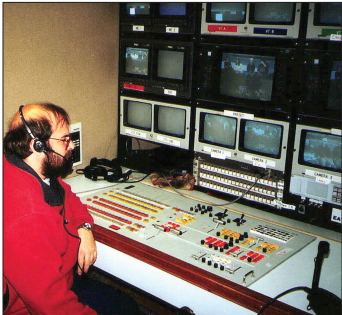
Figure 6.34 By the 1970s, video switcher control panels looked much like they do today. This GVG-1600 switcher was a mainstay on trucks throughout the '80s. This particular switcher has a main program bank and two effects banks, each one associated with a fader bar. The fader bar was used either to do a dissolve, a wipe or a key. A key is just another special type of switch. Whereas wipes are generated by pattern generators in the switcher that determine switching points in the video, video keying circuitry generates switching patterns based on the video being keyed. An internal key uses the video being keyed to generate the pattern, where an external key uses a source that separately generates a key signal, also known as the "whole cut" signal, and the actual keyed video, or fill signal. Each effects bank on this switcher could perform only one operation per bank, either dissolves, wipes or keys. In addition, the path through the switcher was fixed. This meant that each effects bank fed the one below it, but not vice versa, starting with the top effects bank and leading finally
