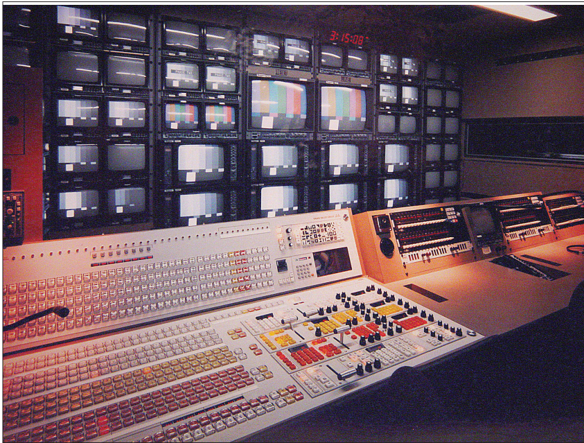
Figure 6.36 A GVG-300 on an ABC truck in the late 1980s. This switcher greatly pushed the state of the art forward. It allowed each bank to perform dissolves, wipes and keys all at the same time. It also was the first to allow random re-entry. This means that there was no fixed cascade from one effects bank to the next. Any effects bank could feed any other. This switcher also had "E-Mem," to remember effects and transitions that could be recalled by an effects bank with a single push of a button. This allowed a larger selection of transitions and effects to be used in a production and allowed the pace of complex visual presentations to increase dramatically. This switcher still had its control panel tightly integrated with the electronics in the actual switching frame. Although there was some serial communications between the panel and the switching frame, there were also many thick cables that went between control panel and frame. (Source: A.F. Associates)
