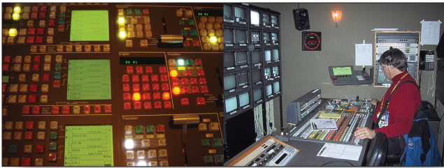
Figure 6.37 Control panels for today's switchers are now really only a user interface that is comfortable to the TD. Unlike earlier switchers, where each button, knob and fader actually had a separate connection back to the switching frame, now the panel interprets what the TD wants to do and via a LAN conversation tells the frame, or tub as it is also known. Control panels over LANs also allow a single control panel to control multiple switching frames. Thus the TD in one truck could control the video switching in two separate trucks. For instance, two different trucks that use different graphics packages, booth cameras, and open, closing and transition "bumpers," but that use the same game cameras, could be controlled by a single TD. (Source: Jason Taubman)
